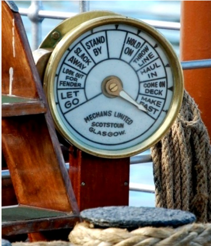
Aft Docking Telegraph on Promenade Deck
